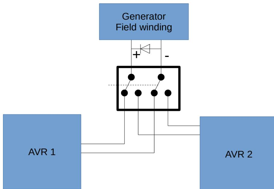
There will be an error message indicating that the system has switched to the second AVR. If the AVRs have a common voltage potential for the field winding, then the relay can possibly be omitted. Please verify before trying.
