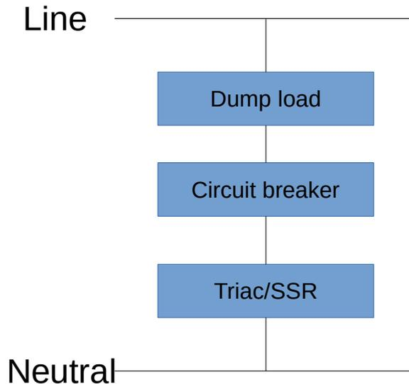
For single phase operation of a 3 phase model, connect only Line 1 dump loads.
